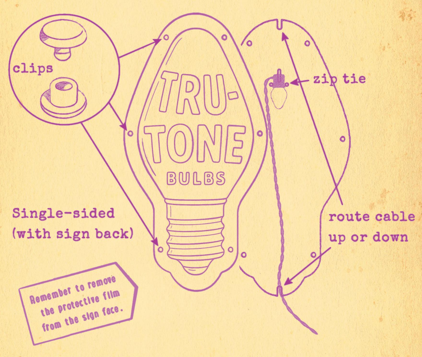
Align the sign face to the sign back, routing the wire through the top or bottom slot (depending on your installation). The included push-to-fit connectors should be snapped together in each of the 6 perimeter holes. The connectors are removable in case you need to access the light bulb.
